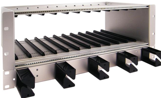
The open chassis 19" 3U allows the cable protection tubes to be fed from the manifold directly to the Compact Module. The anodized aluminium chassis is 84TE and accommodate up to 12 modules.
