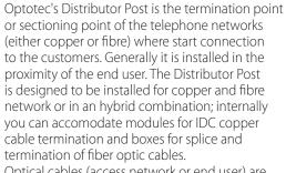
Optical cables (access network or end user) are terminated through the splicing of connectorized patch-cords within appropriate cassettes with a maximum potential up to 24 fibres.
